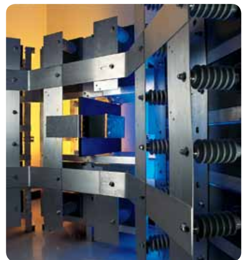
▲ Schneider Electric's lightning generator tests Surgelologic SPDs in real-world systems and situations.
